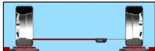
Fig. 23: Measuring of the wheel track
