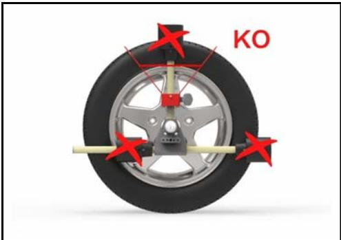
Asymmetrical positioning is wrong, rollers must be positioned approximately in middle of tire shoulder / wall and symmetrical to the center
